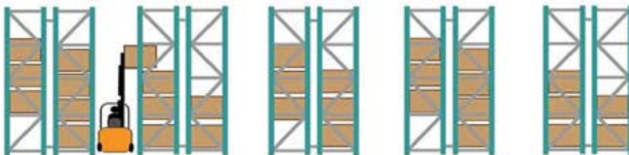
Very Narrow Aisle Rack Configuration
